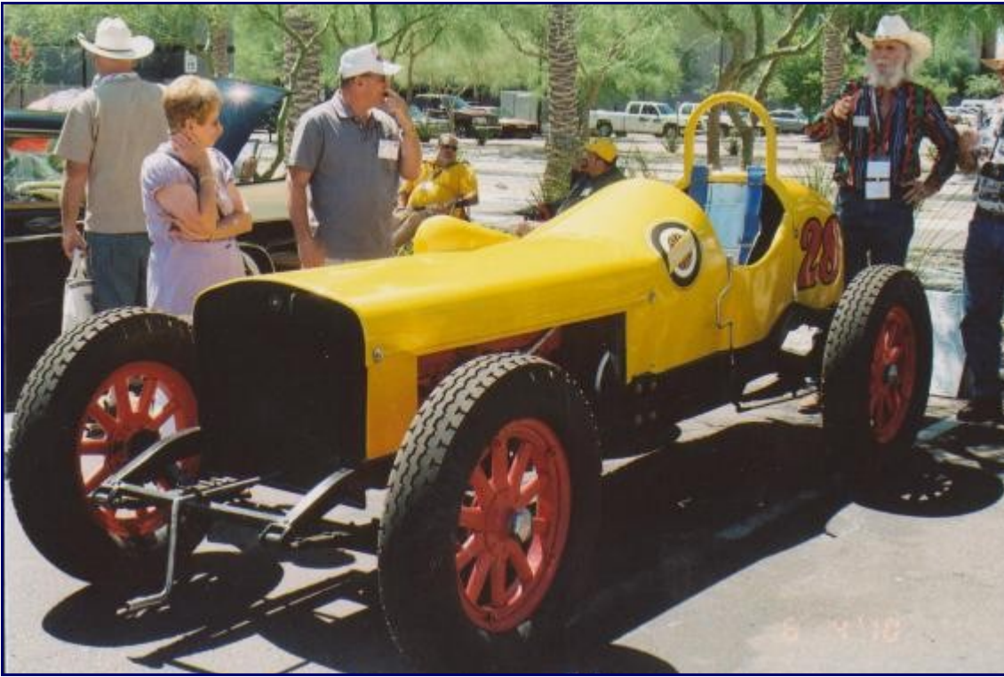
1928 Studebaker President Race Car Constructed from 1920's Studebaker Parts and Fabricated Sheet Metal
